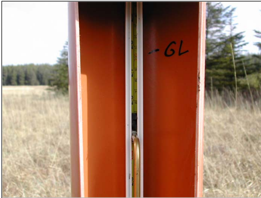
Photograph 2. A close-up of the Walrag pointer area. The height of the pointer is read off the scale (in this case a metal tape measure cut to size) housed in a white plastic moulding. Note the black foam plug at the top of the pointer which provides a measure of the maximum water level reached.
