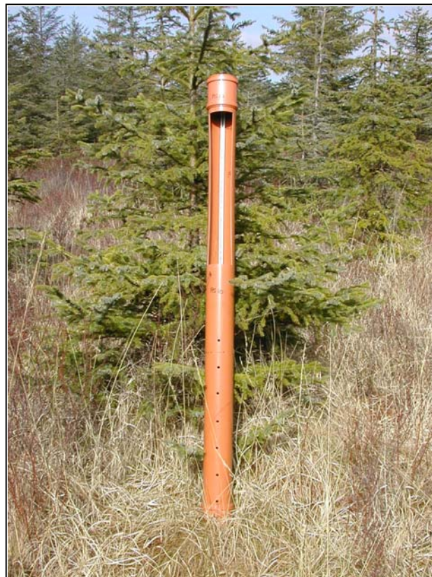
Photograph 1. A Walrag before it is inserted into the peat. Note the holes in the bottom half of the pipe, which allow water into the Walrag.
